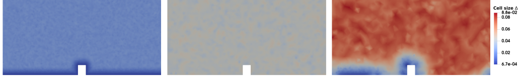
Figure 2: Slice along the y -axis of the ST (left), initial AMC (middle) and final AMC (right) meshes
