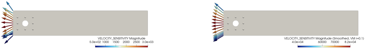
(b) Inlet velocity gradient (on left edge: 14 nodes) for the unsmoothed (left) and smoothed (right) cases.
