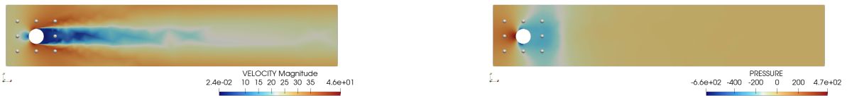
(a) Velocity (left) & Pressure (right) fields of the target solution and location of the 8 velocity and pressure sensors.
