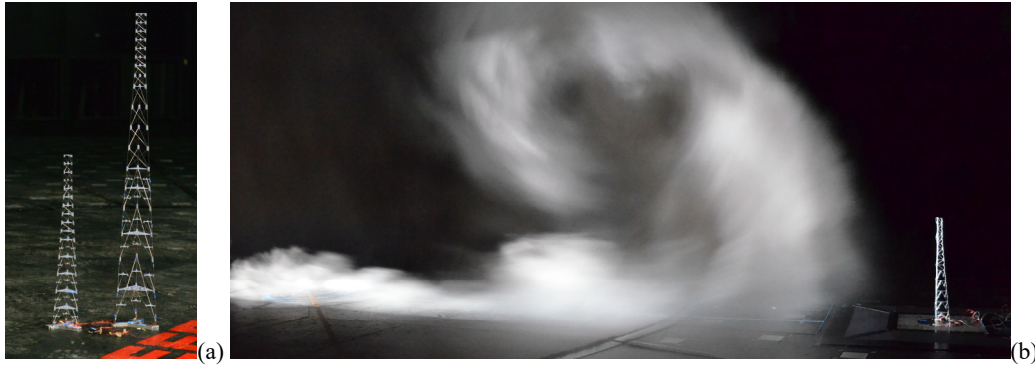
Figure 2: (a) Aeroelastic models of towers T50 (left) and T90 (right) and (b) DB visualization of the T50 model
