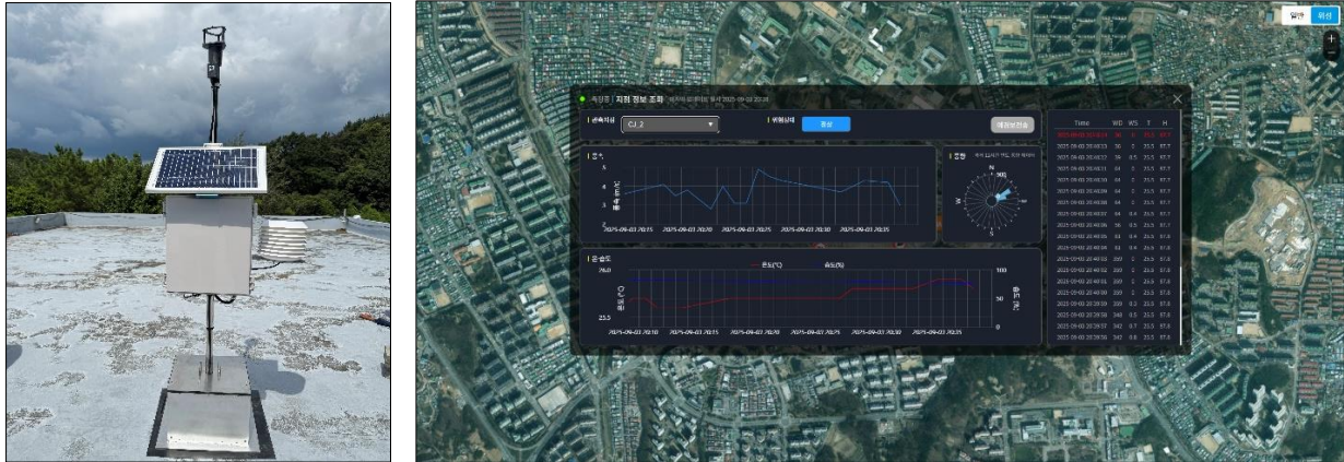
Figure 4: Anemometer and prototype system developed in this study (left: anemometer, right: prototype system)
